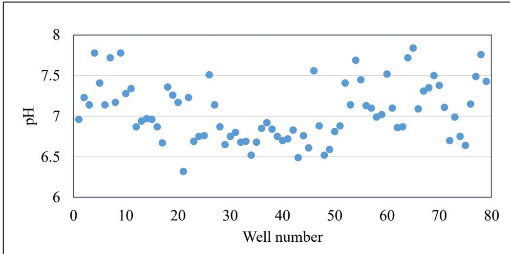
**Figure 2: Variation of pH of well water at different locations of the study area**
