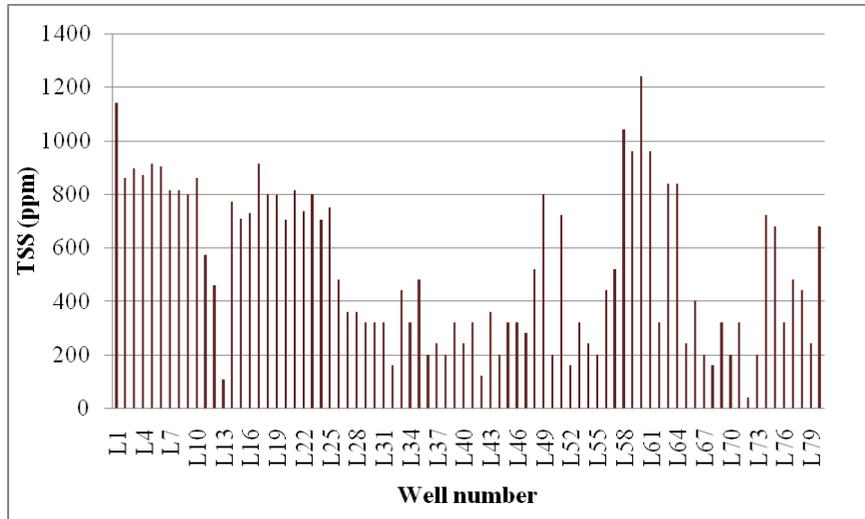
**Figure 4: Total Suspended solids of the well water at different locations in the study area**
