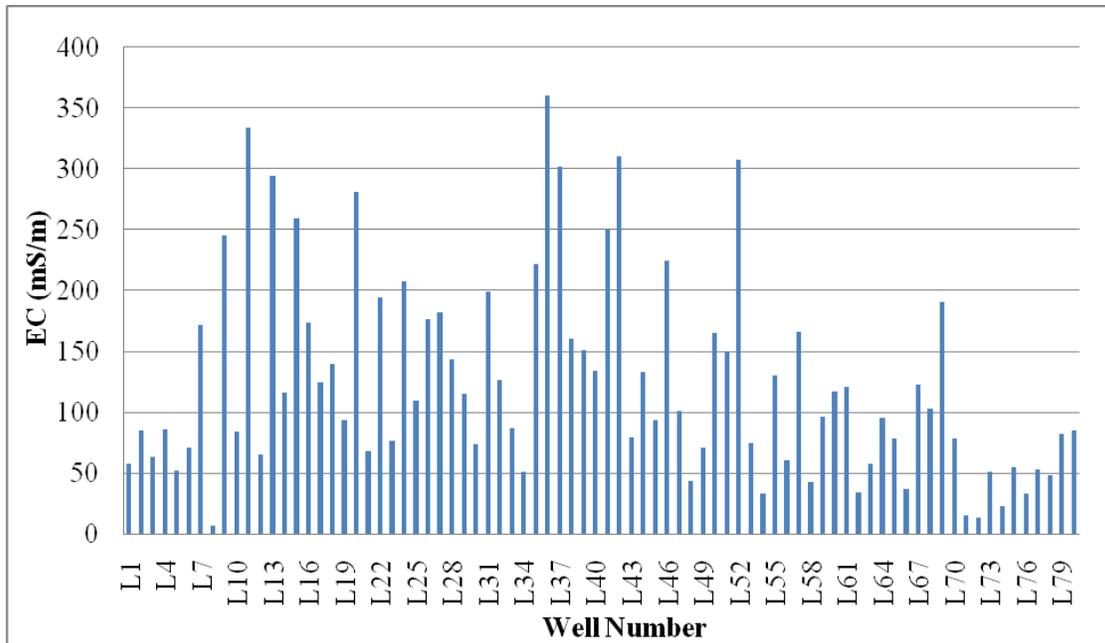
**Figure 3: Electrical conductivity of well water samples in different Locations**
